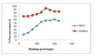
*Figure 4.* Effect of shaking speed (rpm) on MB removal onto RBGH and UMBGH. Adsorbent dose (0.1 g), Time (30 min.), Solution concentration (25 ppm / 50 mL), Temperature (293.0 K)
