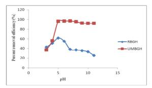
*Figure 6*. Effect of pH on MB removal onto RBGH and UMBGH. Adsorbent dose (RBGH = 0.3g, UMBGH = 0.7 g), Shaking speed (RBGH = 400 rpm, UMBGH = 300 rpm), Solution concentration (25 ppm / 50 mL),Time (50 min.)
