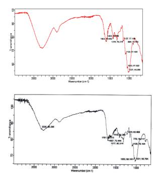
Figure 2. FT-IR spectra of RBGH (before) and UMBGH (after) Urea modification
