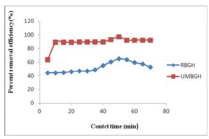
*Figure 5.* Effect of time (min.) on MB removal onto RBGH and UMBGH. Adsorbent dose (0.1 g), Shaking speed (RBGH = 400 rpm, UMBGH = 300 rpm), Solution concentration (25 ppm / 50 mL), Temperature (293.0 K)
